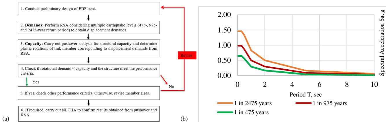
Figure 4 PBD of EBF Bents: (a) design methodology (b) 5% damped Sombrio UHS
