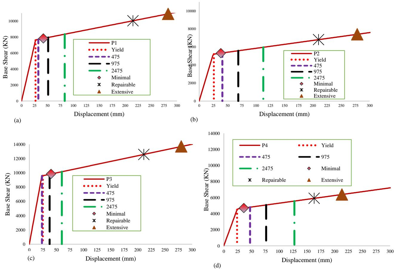
Figure 6 Pushover curves RSA demands and acceptance criteria limits: (a) Design 1, (b) Design 2, (c) Design 3, (d) Design 4
