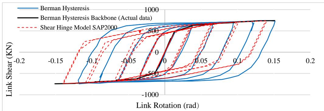
Figure 5 Experimental hysteresis calibration using shear plastic hinge
