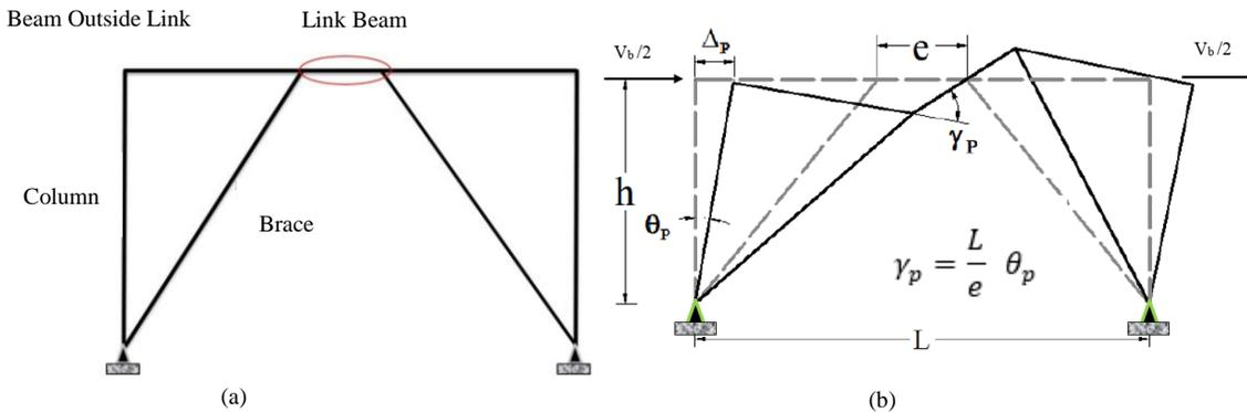
Figure 1 Typical EBF Geometric Configuration: (a) Chevron EBF shape, (b) deformed shape, Adapted from: [3].
