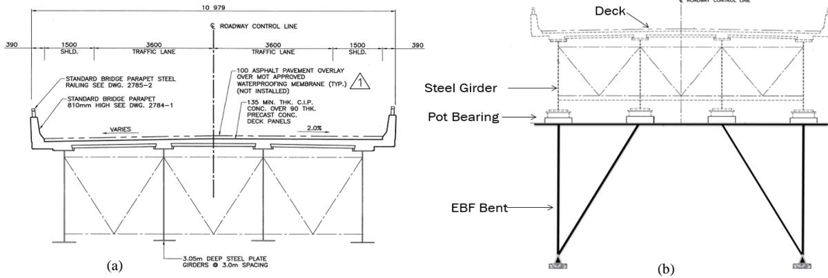
Figure 2 Sombrio Bridge: (a) superstructure typical section [9] (b) replaced EBF bent .
