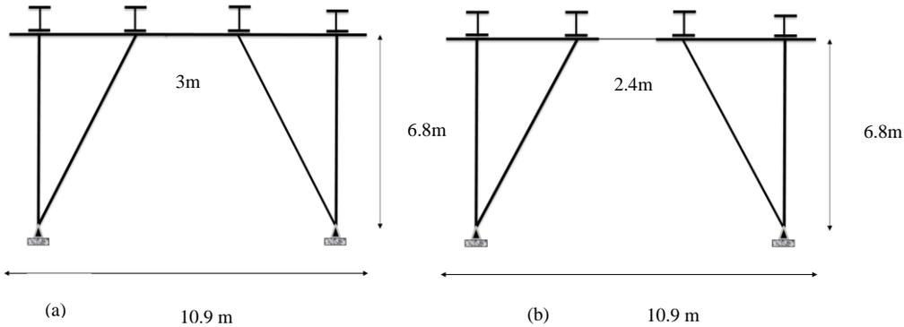
Figure 3 Selected EBF geometry with girders orientation: (a) for design case 1, 2 and 3, (b) for design case 4.
